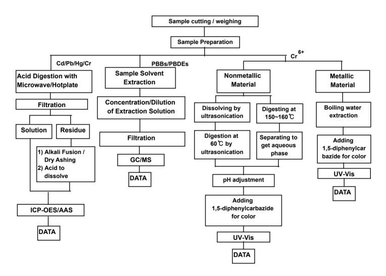
The samples were dissolved totally at the acid digestion step of the above flow chart for Cd,Pb,Hg Section Chief : Timothy Jeon
