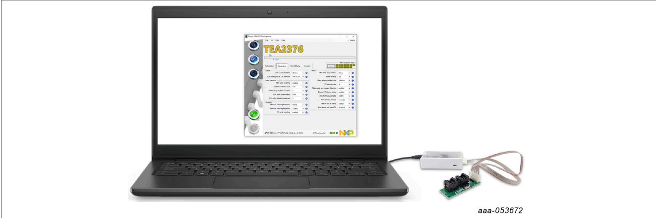
Figure 4. Setup for programming with the Ringo software on a PC
