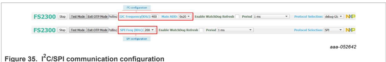
Figure 35. I<sup>2</sup>C/SPI communication configuration
