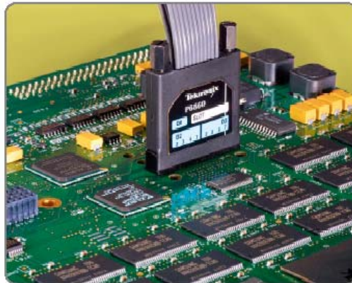
Figure 7-5. Mother Board Connection
