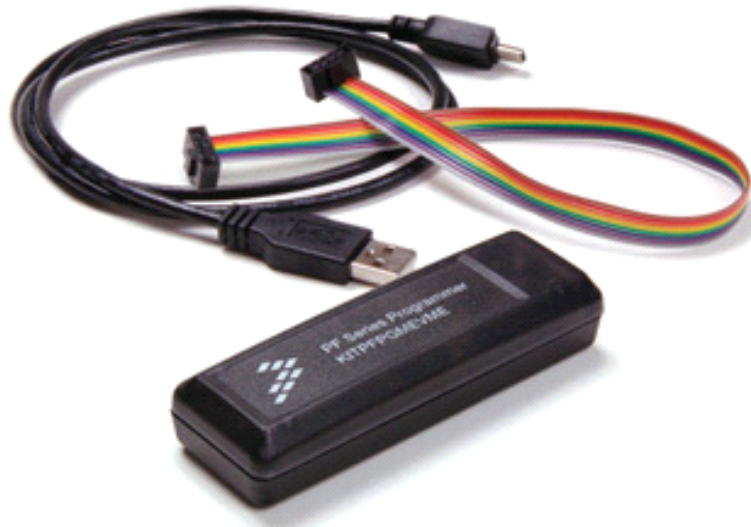
Figure 1. The PF Programmer (KITPFPGEVME)
