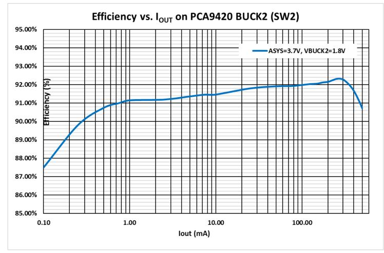
Test Condition: VASYS=3.7V, VBUCK2=1.8V, IBUCK2=0mA to 500mA
