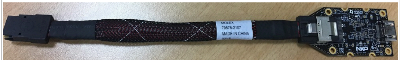
Figure 6. i.MX Mini SAS cable with DSI-to-HDMI adapter IMX-MIPI-HDMI
