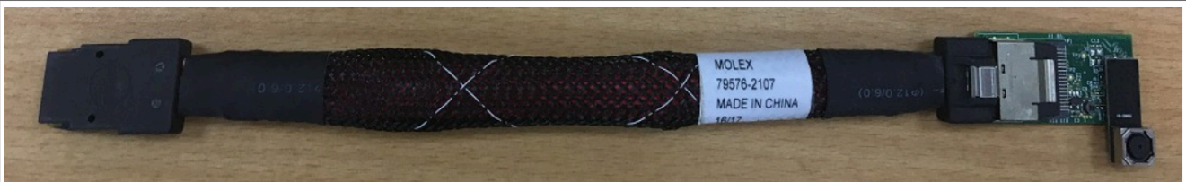
Figure 11. OV5640 CSI MIPI camera
