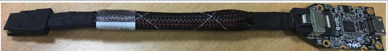
Figure 10. i.MX mini SAS cable with LVDS-to-HDMI adapter
