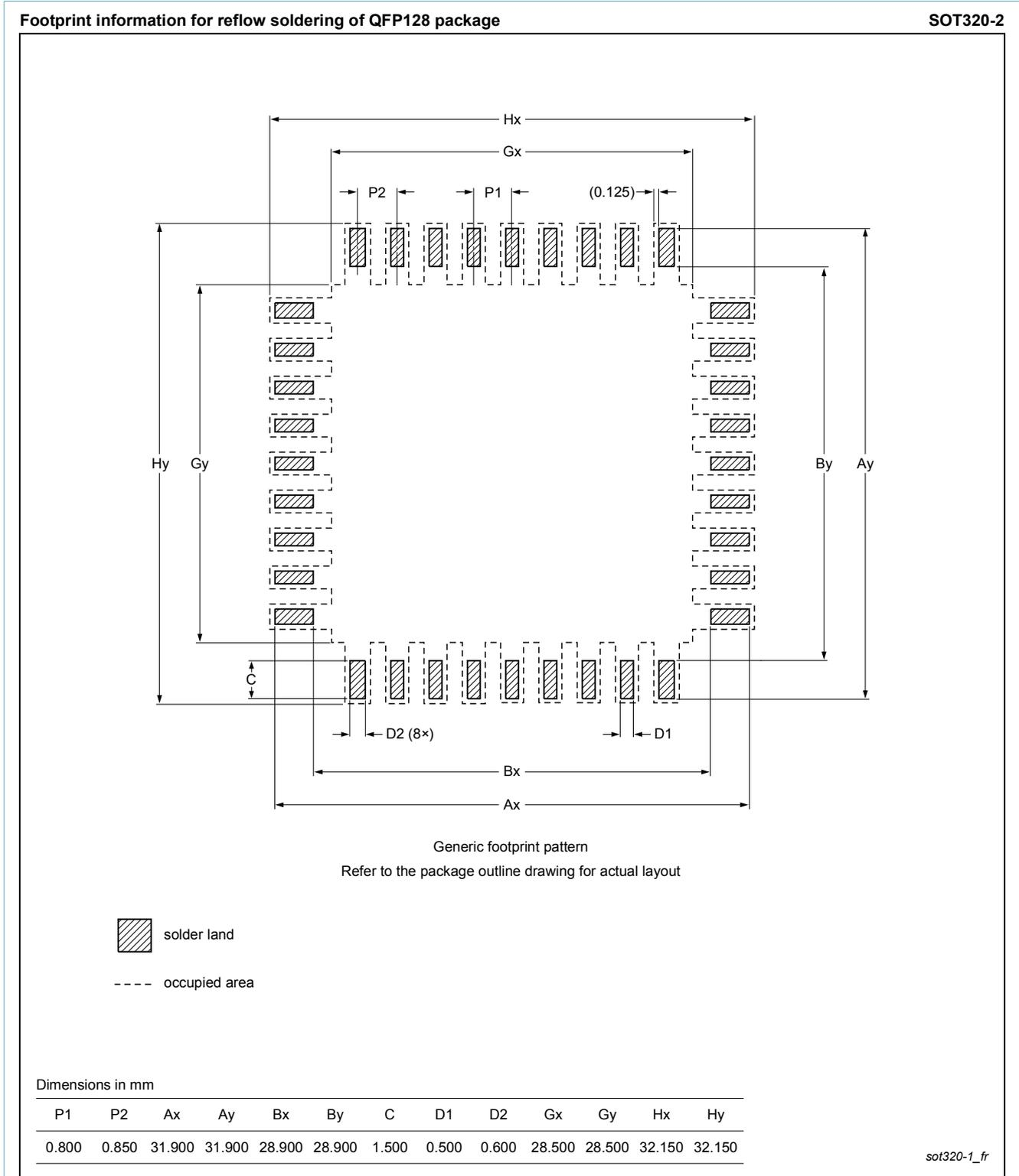
Fig. 2. Reflow soldering footprint for QFP128 (SOT320-2)
