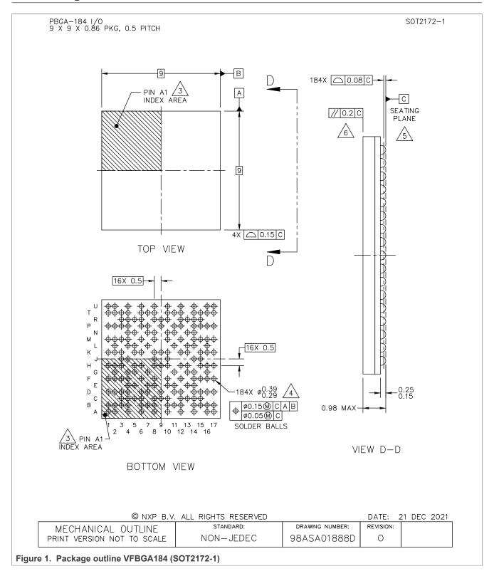
VFBGA184, very thin fine-pitch ball grid array package, 184 terminals, 0.5 mm pitch, 9 mm x 9 mm x 0.86 mm body
