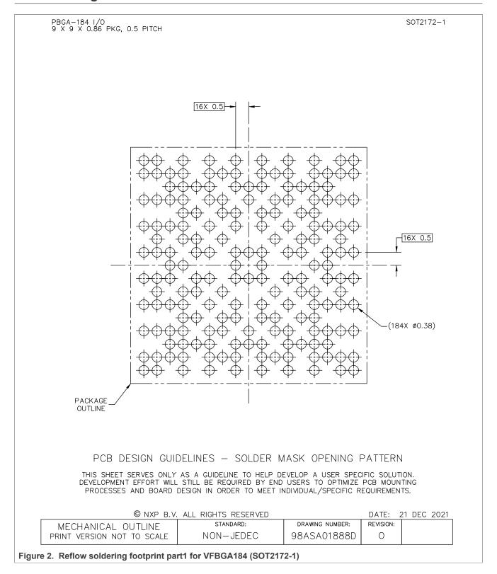
VFBGA184, very thin fine-pitch ball grid array package, 184 terminals, 0.5 mm pitch, 9 mm x 0.86 mm body
