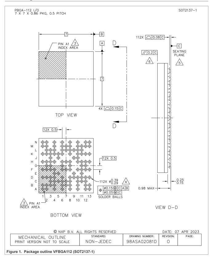
VFBGA112; very thin fine-pitch ball grid array, 112 terminals, 0.5 mm pitch, 7 mm x 7 mm x 0.86 mm
