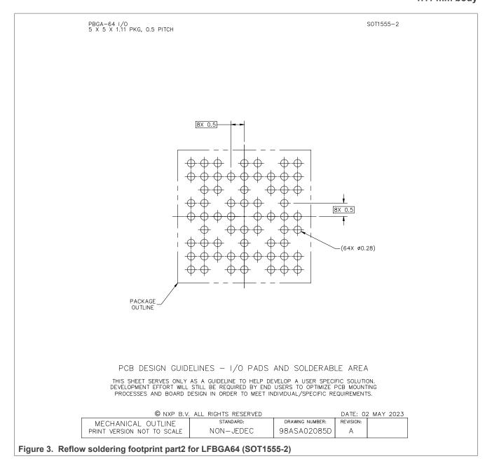
LFBGA64, plastic, low profile fine-pitch ball grid array; 64 bumps; 0.5 mm pitch; 5 mm x 5 mm x 1.11 mm body
