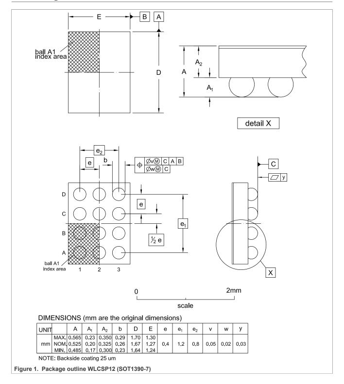
WLCSP12, wafer level chip-scale package; 12 bumps; 1.67 mm x 1.27 mm x 0.525 mm (backside coating included)
