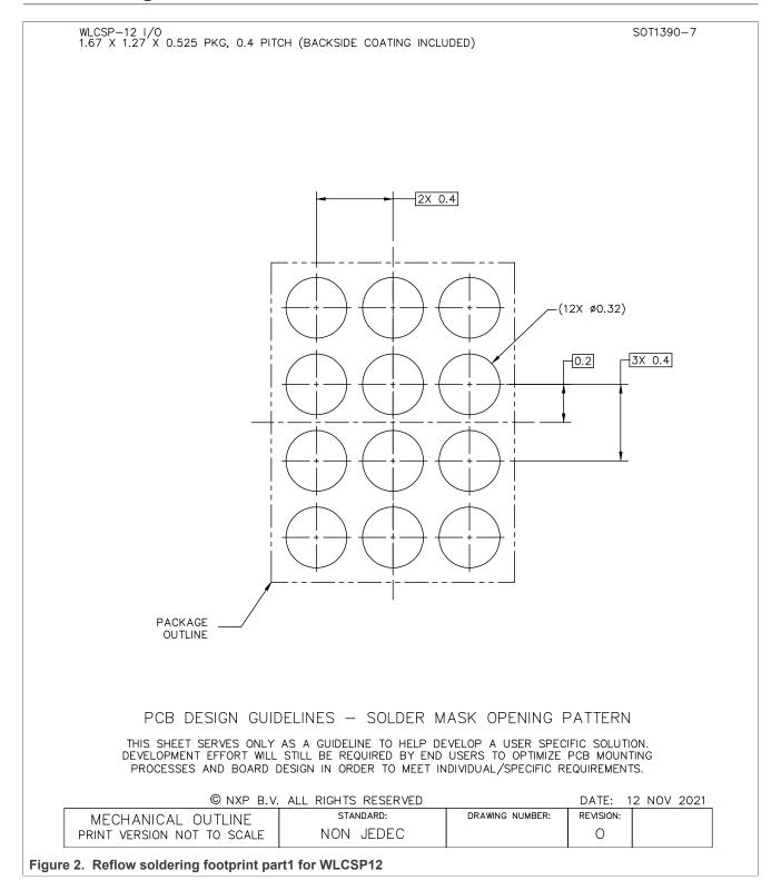
WLCSP12, wafer level chip-scale package; 12 bumps; 1.67 mm x 1.27 mm x 0.525 mm (backside coating included)
