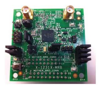
Typically the 12311-MRB mounts on TWR-RF for power and control, partially visible in photos below.
