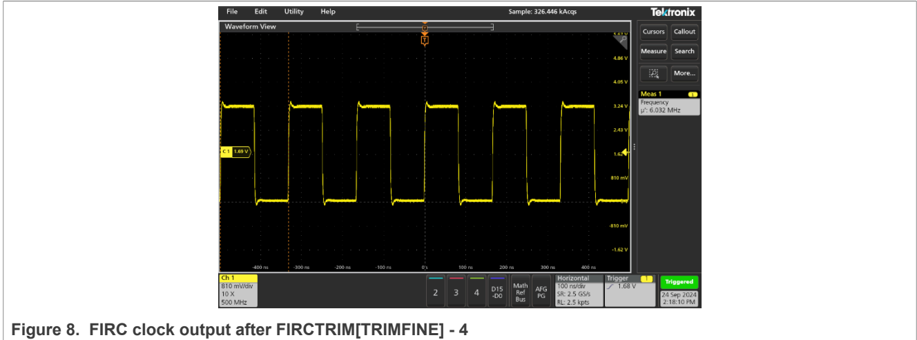
Figure 8. FIRC clock output after FIRCTRIM[TRIMFINE] - 4
