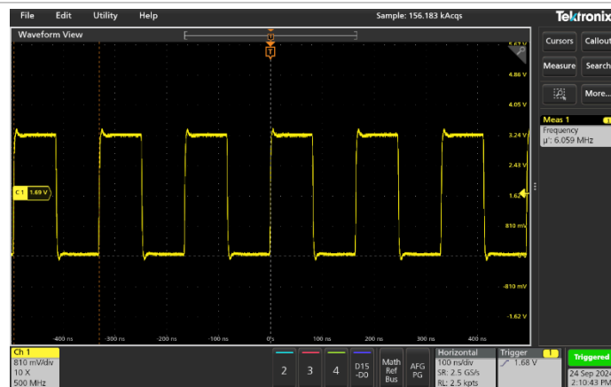
Figure 7. FIR clock output after FIRCTRIM[TRIMFINE] + 4
