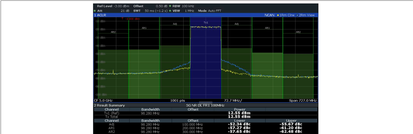
Figure 17. BTS6305C ACLR DPD versus none-DPD at 5.0 GHz center frequency and P out = 12.5 dBm, CF = 10 dB
