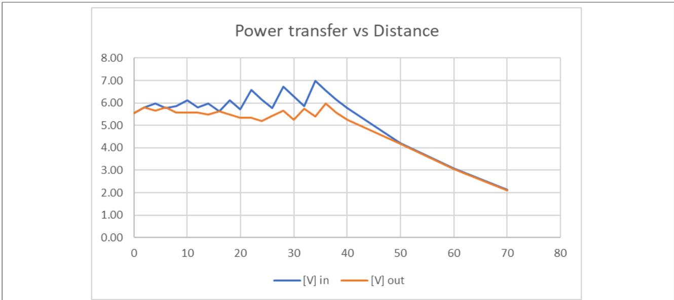
1. Distance in mm, power transfer in V, measured at the EMVCo 2.6 TestPICC
