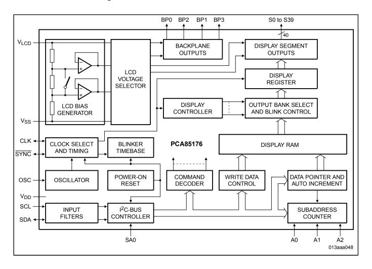
View additional information for 40 X 4 Automotive LCD Driver for Low Multiplex Rates.
