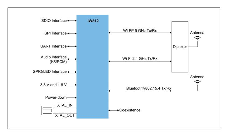
View additional information for 2.4/5 GHz Dual-Band 1x1 Wi-Fi® 5 (802.11ac) + Bluetooth® 5.4 + 802.15.4 Tri-radio Solution.
